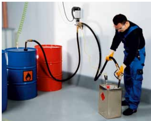
Filling of solvents from a 200 litre drum into different containers.
