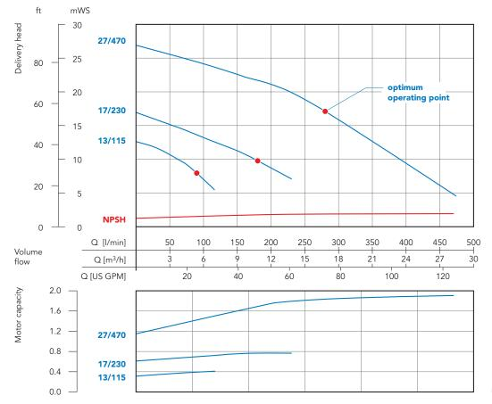
Determined with water of 20 °C; measured values  $\pm$  10%
