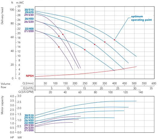
Determined with water of 20  $^{\circ}\text{C};$  measured values ± 10 %
