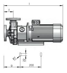
Fig.: MA pump type 6 with motor of up to 2.2  $\rm kW$
