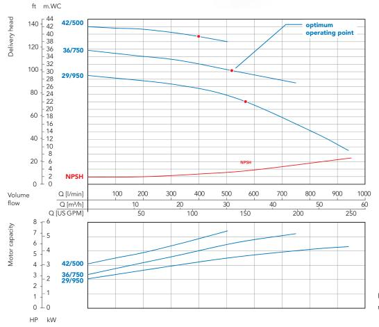
Determined with water of 20 °C; measured values  $\pm$  10%
