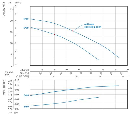
Determined with water of 20 °C; measured values  $\pm$  10 %
